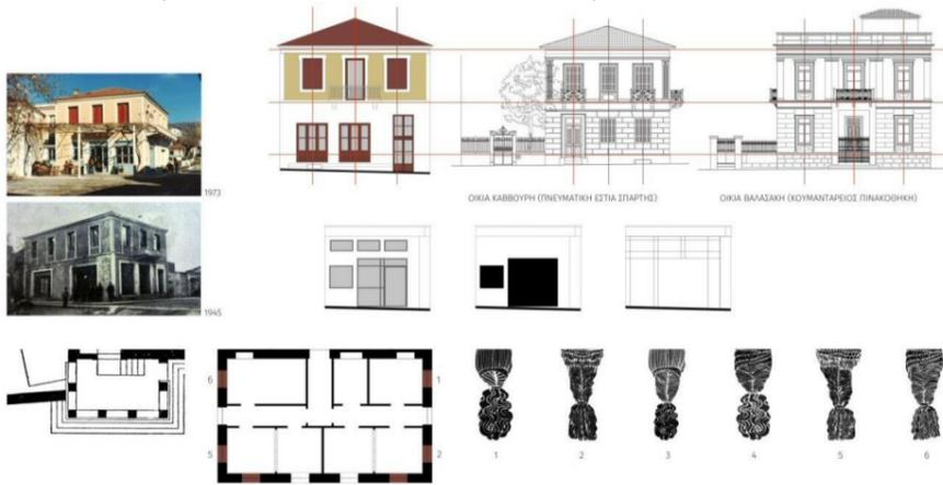
More specifically: ♦ The auxiliary spaces of the ground floor shopping centre intended for rent are re-adapted and re-constructed in a uniform, consistent way. ♦ In the same area, we take advantage of the height of the space and put into suspended ceilings the necessary mechanical heating, cooling and ventilation installations.
