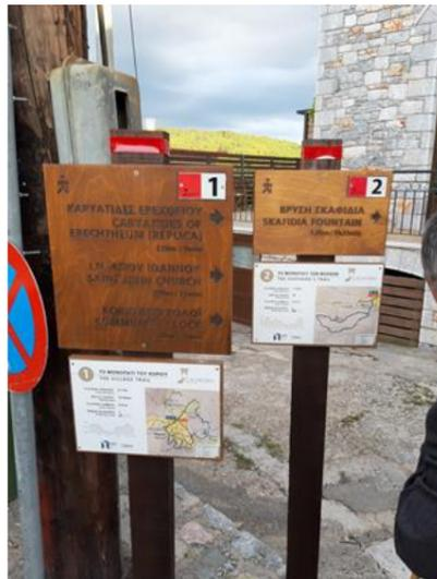
It should be noted that an innovation was applied to the signs: wooden niagon stakes with three layers of impregnation with protective varnish on the entire surface and two layers of asphalt insulating material at the base of the piles for absolute protection from soil moisture.
